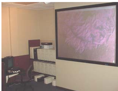
Figure 12. Front projection, polarization-preserving white screen.
