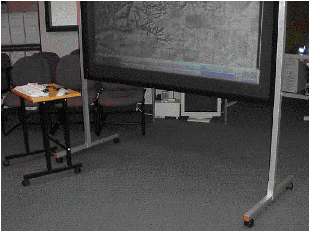
Figure 13. The portable, rear-projection, polarization-preserving black screen.
